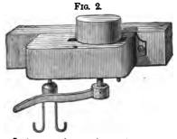
Instrument for causing croisseur, scale a natural size; not now used, twisting-in the croisseur by hand preferred.
