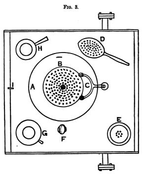
Tray and utensils of cocoon reeling frame ; mechanical drawing, scale 1 inch to the foot.
