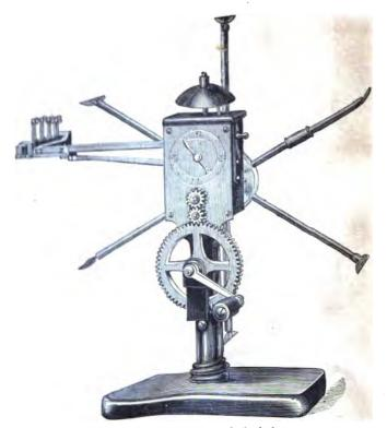
Deniering and measuring reel; scale { of the real size. COCOON REELING.
