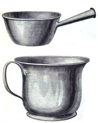
Brass vessels belonging to tray of cocoon reeling machine ; scale  $\frac{1}{2}$  of the real size. COCOON REELING.
