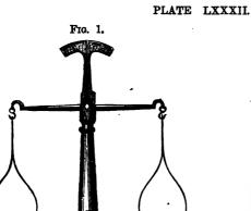
Fine balance for deniering; scale  $\frac{1}{5}$  of real size.
