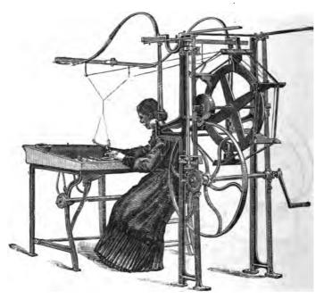
European Cocoon-reeling machine, diagonal view, System Chambon (French).
